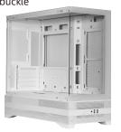
Disassemble the right side panel from back buckle
